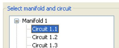
Circuit named *Circuit1.1* is selected in the example above. Now the dialog displays the circuit information, which can be edited by the user. The selections can be accepted with *OK* or discarded with *Cancel*. Here you can also select another manifold or circuit that you want to edit.
