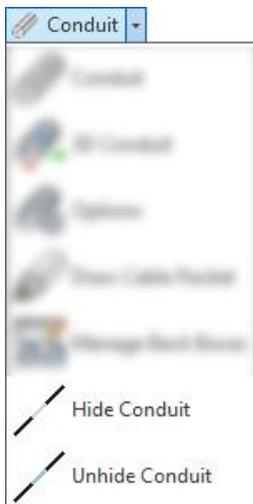
When using the "Hide Conduit" function, you need to show two points from a conduit segment and the segment will be hidden in the current view between those points by utilizing special union fittings and splitting the segment into pieces. The function continues as long as you press Esc.
