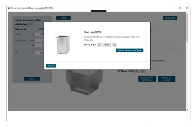
5. Import to MagiCAD -button starts the insert operation. Dimensio window is closed and Insert Roof Cowl view is displayed:
