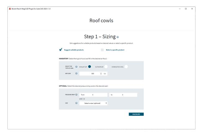
2. Proceed by selecting the wanted type of the cowl (exhaust, outdoor, combination cowl) and enter the required airflow and other wanted search parameters. Optionally you can choose to size a specific product, which allows you to directly choose from list of available products within the cowl type. After that click the calculate -button, and Dimensio will show list of suitable products:
