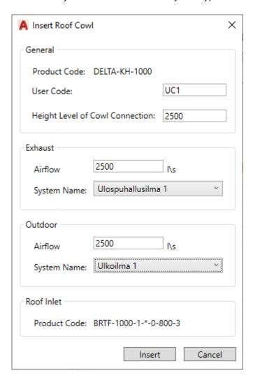
Plugin creates additional connector to the outdoor system in case of combination cowl:
