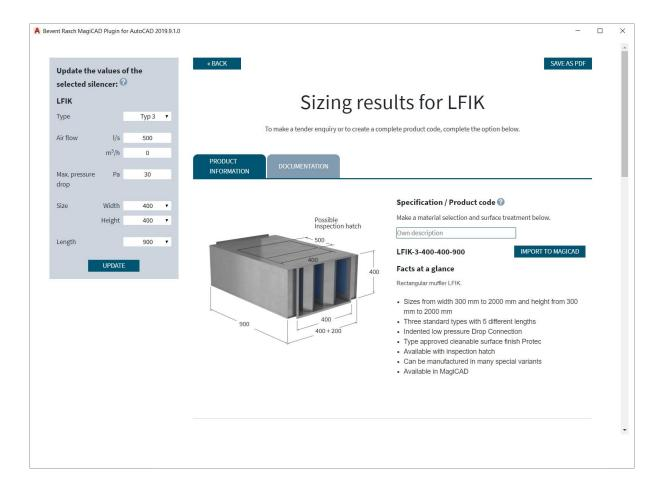
6. From product view click Import to MagiCAD -button in order to insert the silencer into MagiCAD project. Once the button is clicked, Dimensio window is closed and MagiCAD User Code dialog is loaded:
