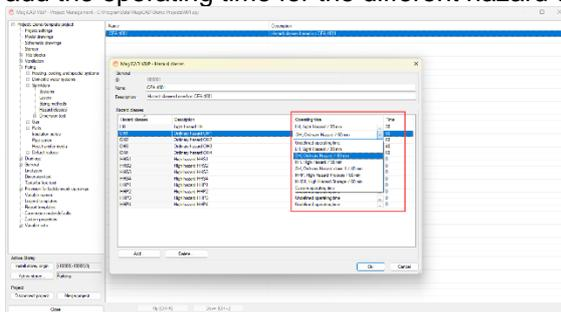
When the sprinkler calculations are run the report will show the selected Operating time as well as the suggested tank size, based on the flow and the operating time:
