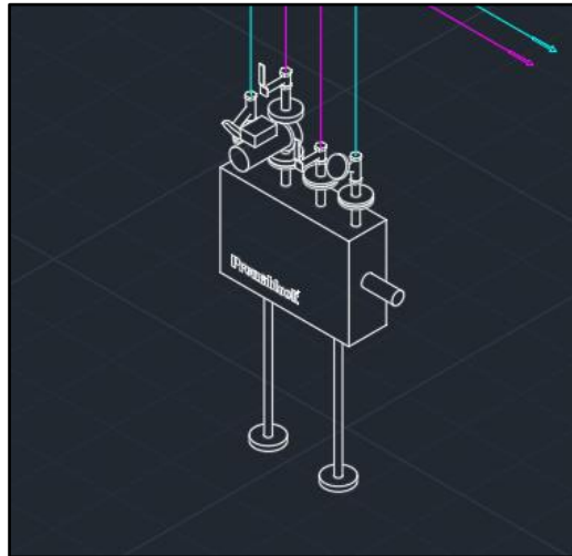
Figure 9 Shunt unit inserted to MagiCAD and connected to primary and secondary circuits
