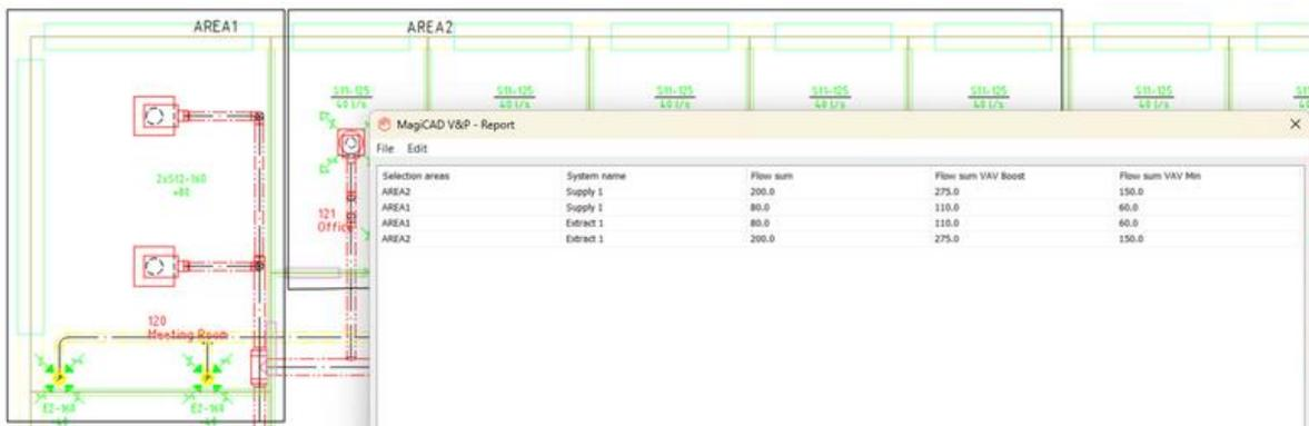
**Note:** If a device is not a VAV-device, then the VAV min and VAV boost flows will be 0.
