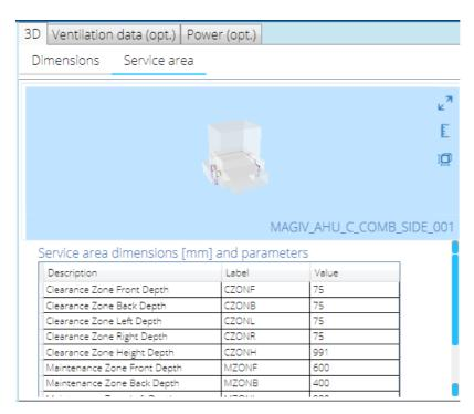
The **Service area** sub tab only exists with parameters starting with "**CZ**" or "**MZ**" in the 3D Geometry.
