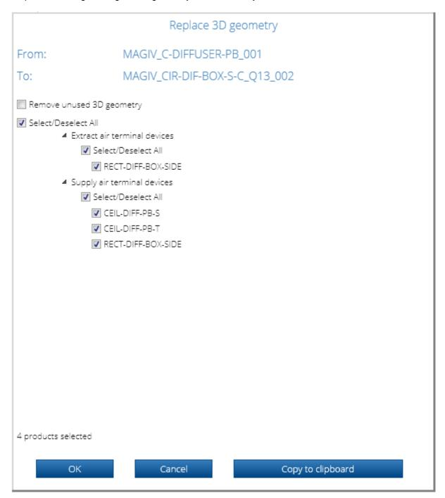
If all products are selected, the unused 3D geometry can be removed by checking the **Remove unused 3D geometry** checkbox.
