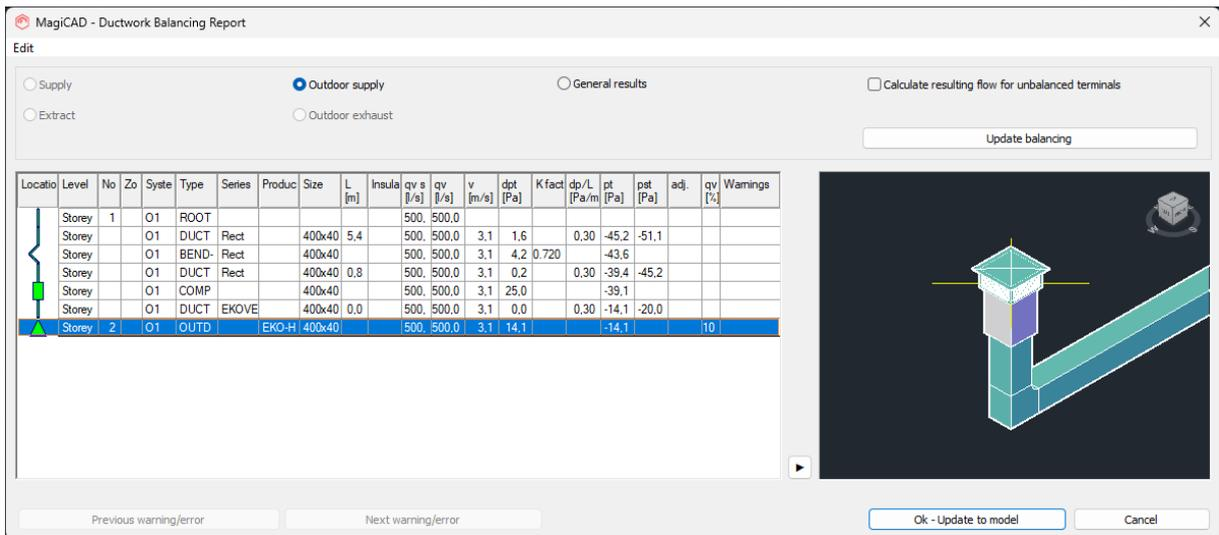
Figure 15 MagiCAD Ductwork balancing report
