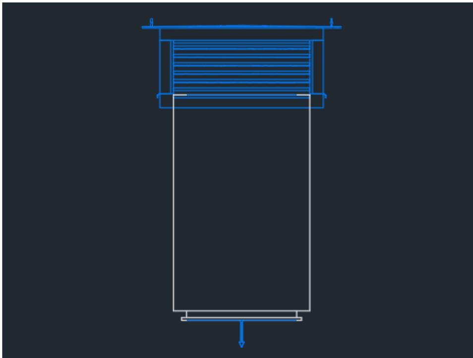
Figure 13 Outdoor supply roof hood and inlet products 3D geometry in AutoCAD drawing
