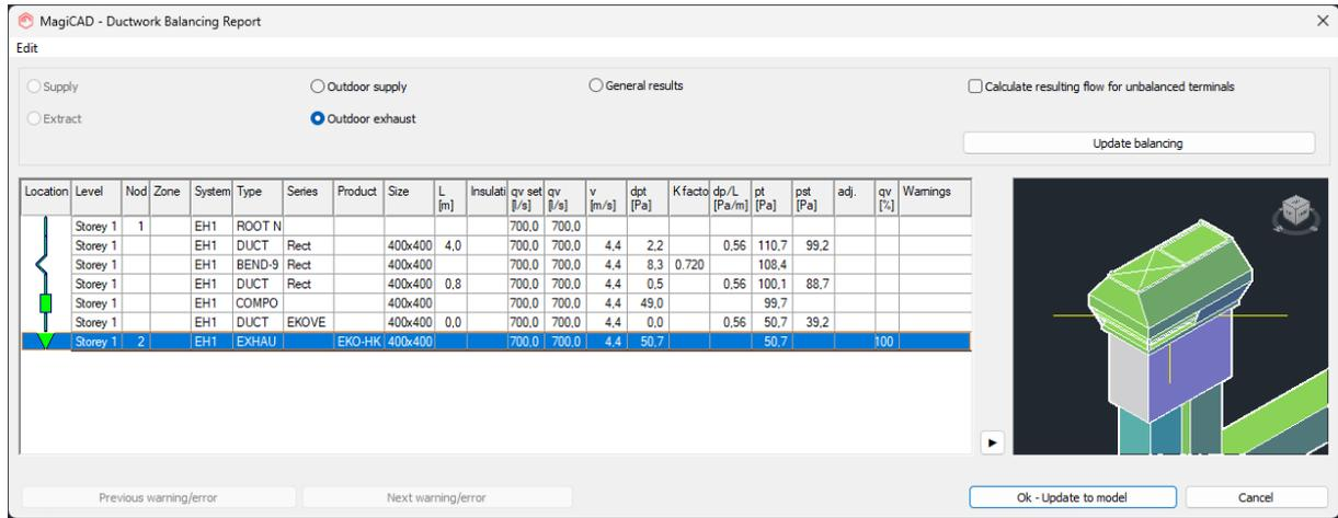
Figure 23 MagiCAD Ductwork balancing report for exhaust part
