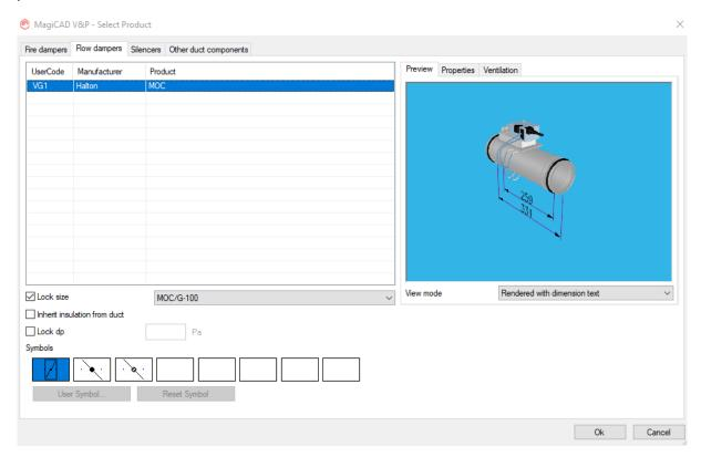
6. After clicking *Ok* button from the dialog, the user can insert the selected product into a duct by clicking on the desired spot.
