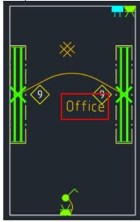
New information fields for cable trays, conduits, lighting tracks, busbar and LED-stripes Type name have been added to cable trays, conduits, lighting tracks, busbars and LED-stripes. Material code and Material name have been added to cable trays and conduits.
