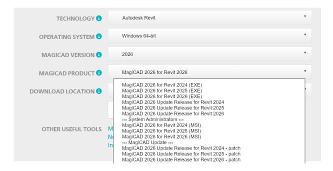
With Update Releases, when updating your existing installation, you have the option to download the relevant installation package directly via MagiCAD's Check for Updates function.
