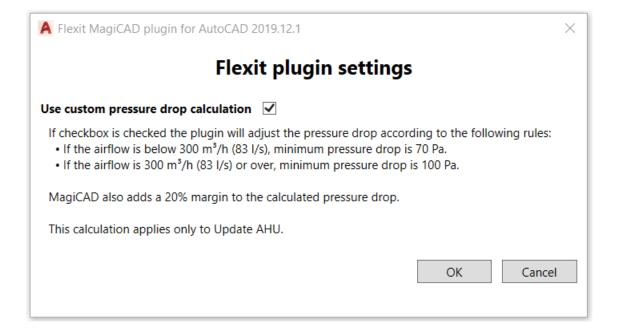
2. To use the custom pressure drop calculation click on the checkbox.
