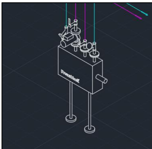
Figure 8 Shunt unit inserted to MagiCAD and connected to primary and secondary circuits
