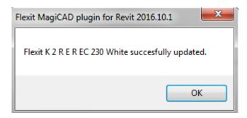
In case the air handling unit has been changed somehow (or switched to a completely another one), the plugin performs replace operation. In the replace operation the plugin deletes the original air handling unit from the drawing and places a new unit to the same position with the same system selections. The following dialog is displayed to the user:
