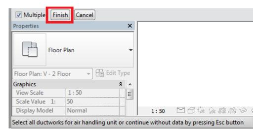
The ducts can be seleced with Revit multiselection tool or one by one.
