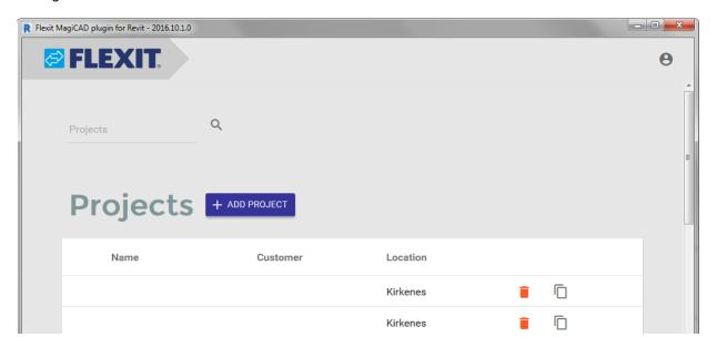
The user can add a new project from this page. After the project is added, the user can continue to add an air handling unit (or units) to project.
