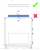
In these cases, the duct component must be inserted to the side of the air handling unit and moved into place after the insert operation.
