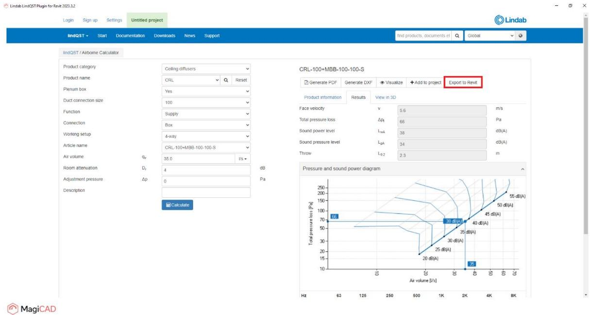
In Airborne calculator proceed by making the required input and then calculate the product. After that proceed by clicking the Export to Revit -button in order to insert the product to Revit.
