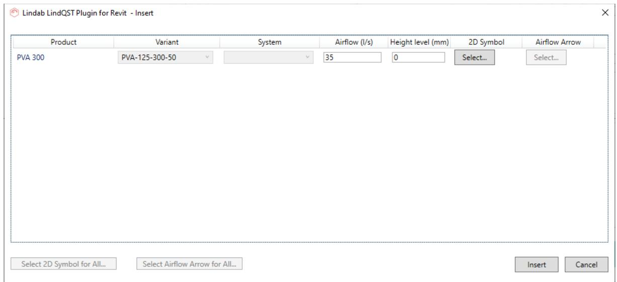
The 2D symbol can be selected for the silencer by clicking the 'Select...' button in the 2D symbol column:
