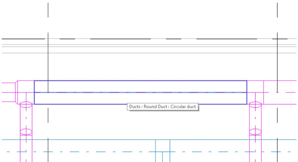
8. LindQST damper calculator is opened. If you selected the duct in Revit, information read from it is now populated automatically into corresponding fields in LindQST (fields highlighted in red):
