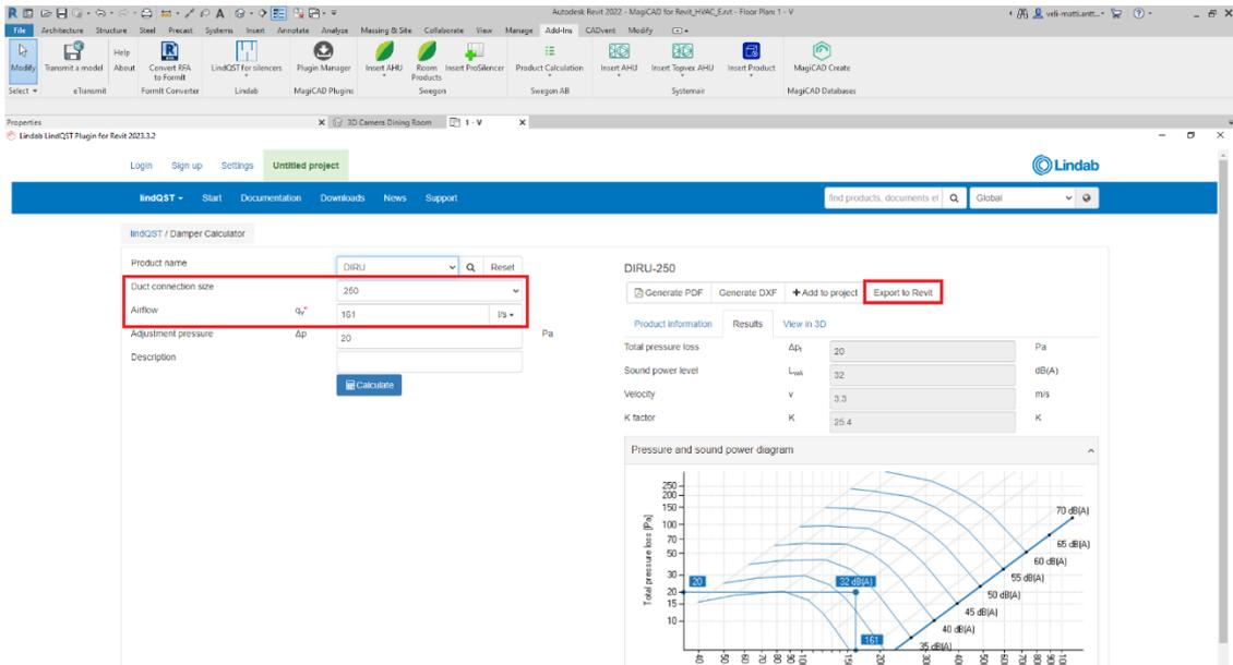
9. Proceed by selecting the wanted product and calculate it. Then click Export to Revit -button in order to insert selected damper into Revit project.
