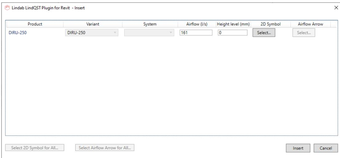
2D symbol can be selected for the damper by clicking the Select... -button from 2D symbol column:
