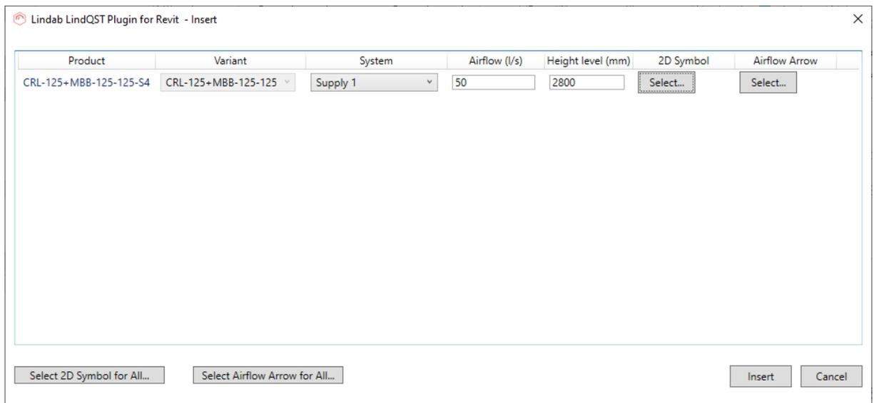
Proceed by making required system selections, set height level and select suitable 2D symbol and airflow arrow for the product.
