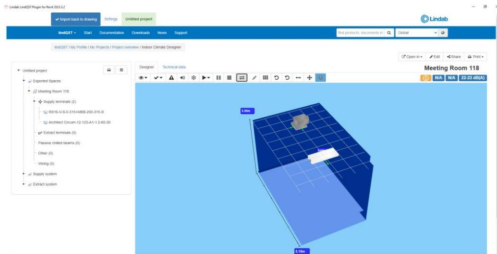
10. User can add more products to the room or modify the existing ones if needed. Once modifications to the products have been made, updates can be sent back to Revit by clicking the Import back to drawing -button.
