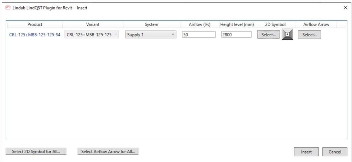
Airflow arrow can be selected for airborne products with similar steps by clicking the Select... - button from Airflow Arrow -column.
