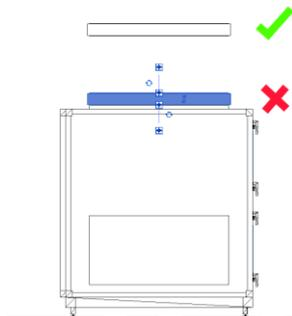
In these cases, the duct component must be inserted to the side of the air handling unit and moved into place after the insert operation.
