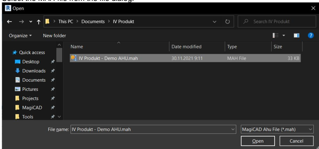
3. After clicking the *Open* button, the plugin reads the transfer file (\*.MAH) and loads the air handling unit(s) to the installation dialog.
