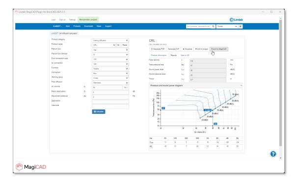
In Airborne calculator proceed by making the required input and selections and then calculate the product. After that proceed by clicking the Export to MagiCAD button in order to insert the product to MagiCAD.
