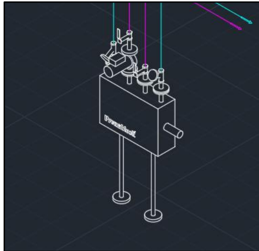
Figure 8 Shunt unit inserted to MagiCAD and connected to primary and secondary circuits
