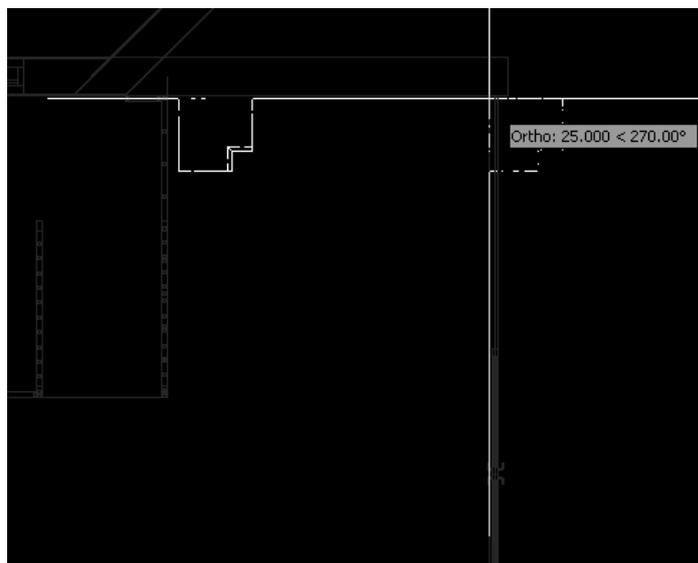
Connect two corner elements together by adding horizontal element between them. Same way it is possible to add horizontal element between corner and connect element. When inserting horizontal element user is asked to select two elements and then horizontal elements is drawn between selected elements as long as the two elements have been aligned properly.
