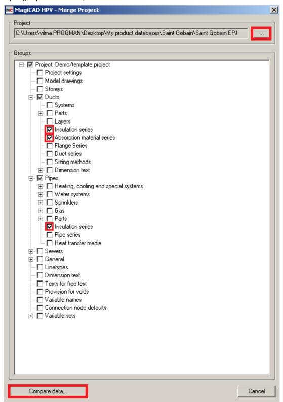
In the opened window you can see all *Insulation series* and *Absorption material series* that will be added to the current project. Choose *OK – Merge* button.
