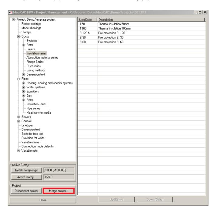
In the opened window choose the project (.EPJ file) from where you have saved it. Choose duct *Insulation series* and *Absorbtion material series* under the Ducts group and pipe *Insulation series* under Pipes group. Choose Compare data...
