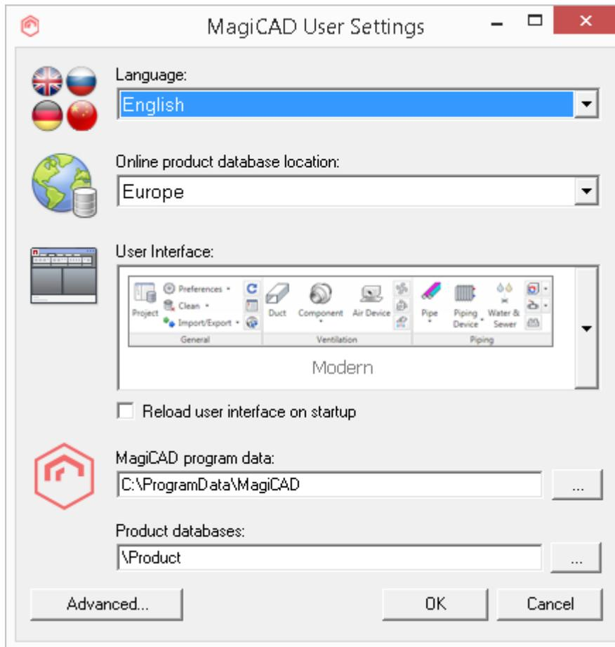
The “User Settings” utility can be started any time after installation from its shortcut in “*MagiCAD / MagiCAD for AutoCAD – Utilities*” folder on the desktop. MagiCAD also checks if the settings are made for the current version, and if the user settings utility has not been run yet, starts the utility.
