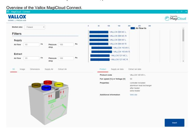
When the *Insert AHU* feature is started from the Vallox MagiCloud Connection, the user is asked to select duct connections from the current view. The user can also continue without selecting the duct connections.
