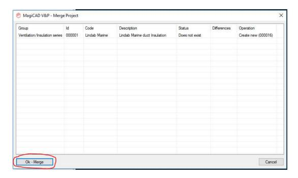
New insulation series are added to the current project file and can be used in the drawing.
