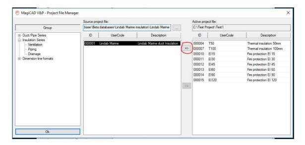
New duct insulation series are added to the current project file and can be used in the drawing.
