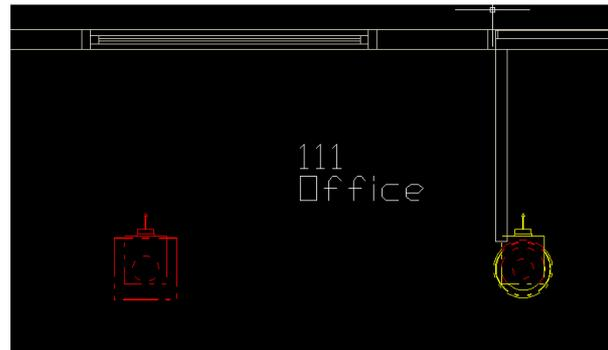
If you don't have the MagiCAD Room module you must draw the rooms boundaries manually using the AutoCAD Polyline function.
