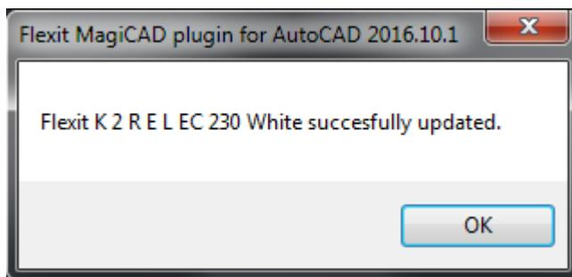
In case the air handling unit has been changed somehow (or switched to a completely another one), the plugin performs replace operation. In the replace operation the plugin deletes the original air handling unit from the drawing and places a new unit to the same position with the same MagiCAD system selections. The following dialog is displayed to user:
