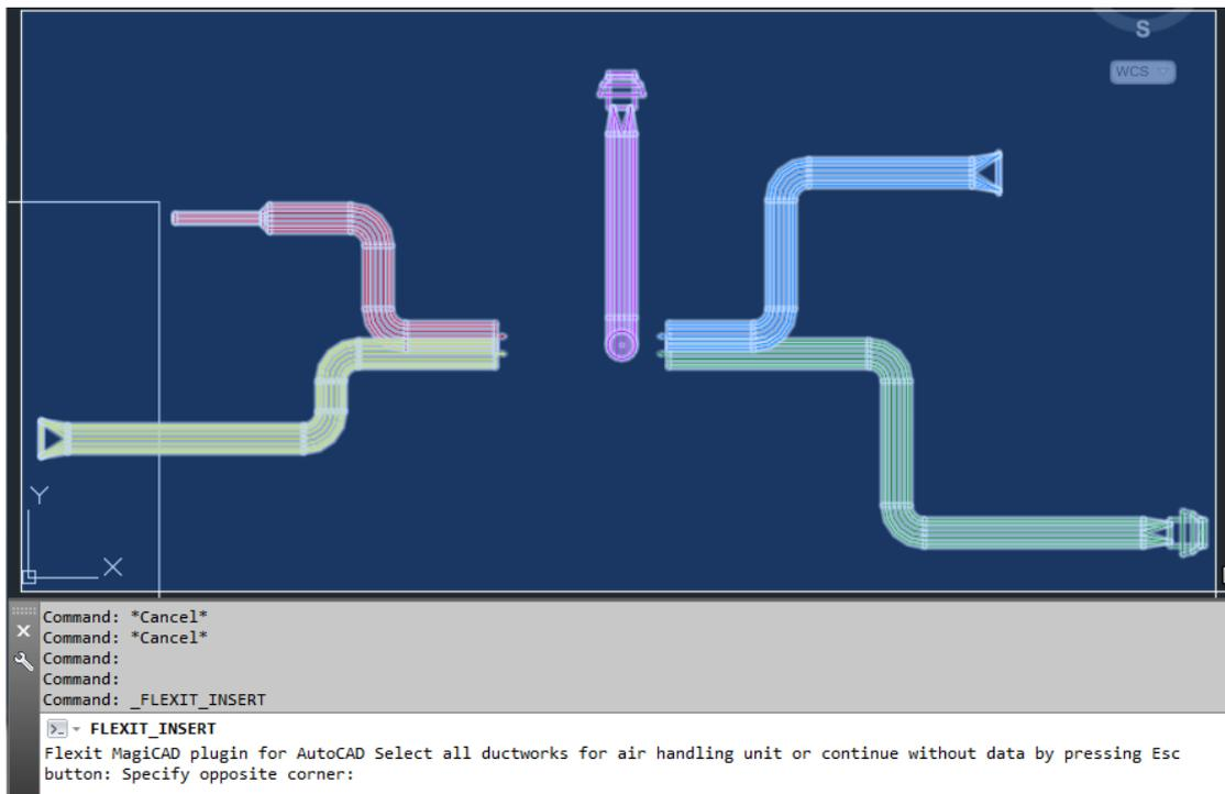
The ducts can be selected with AutoCAD multiselection tool or one by one.
