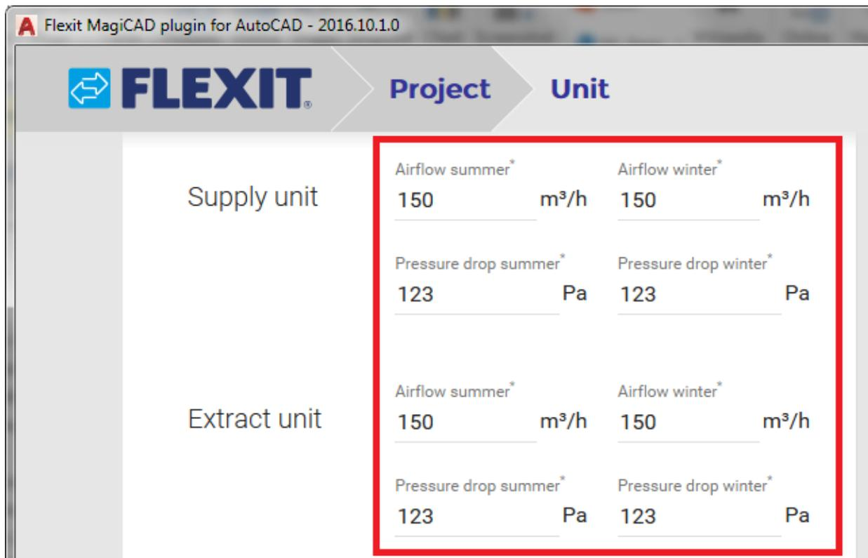
The user can change the predefined air handling unit type or edit unit properties from the *Unit* page.
