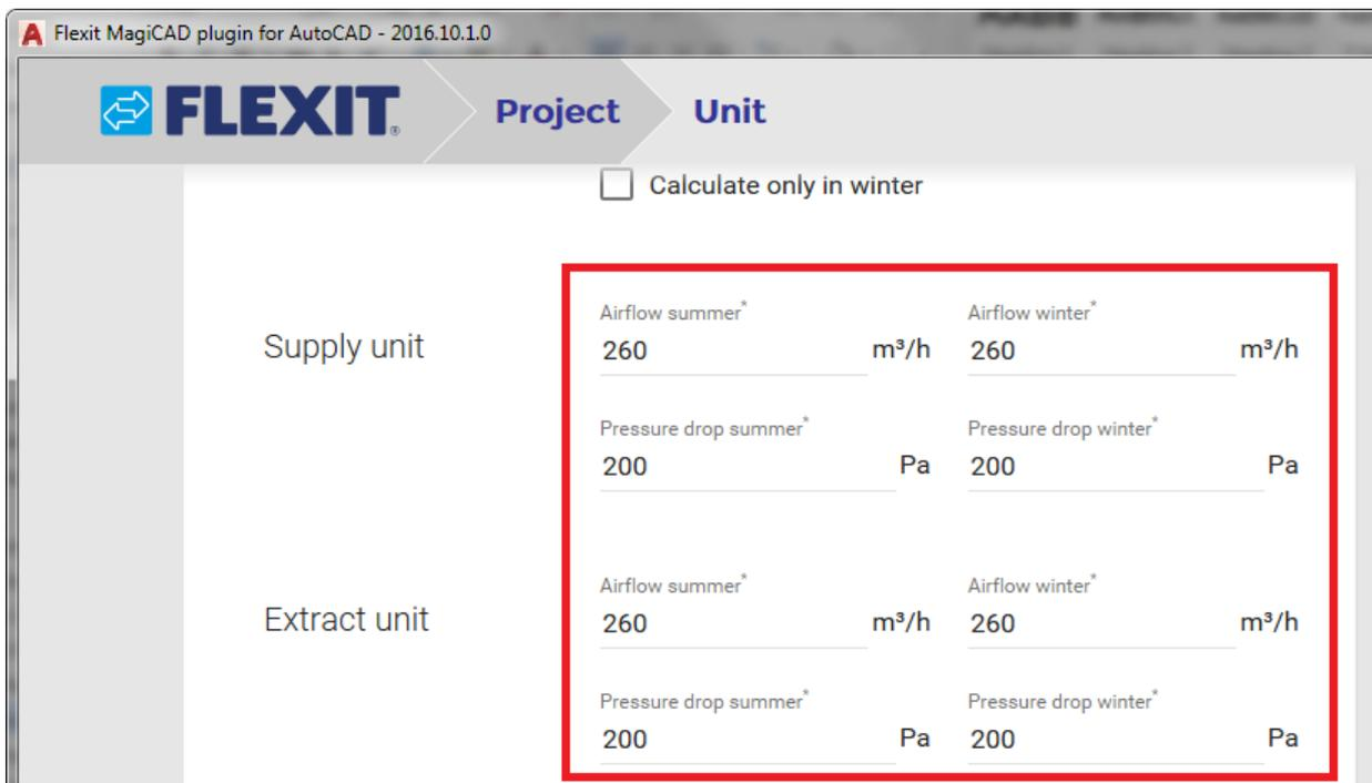
The user can change the predefined air handling unit type or edit unit properties from the *Unit* page.
