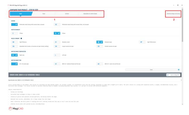
2. User can configure the different aspects of the product from the tabs (1). Technical values can be configured in the "Technical design and sizing" tab (2).
